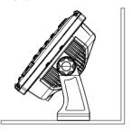
3: Make sure the display can be adjusted to the correct angle without interfering with the surrounding.
